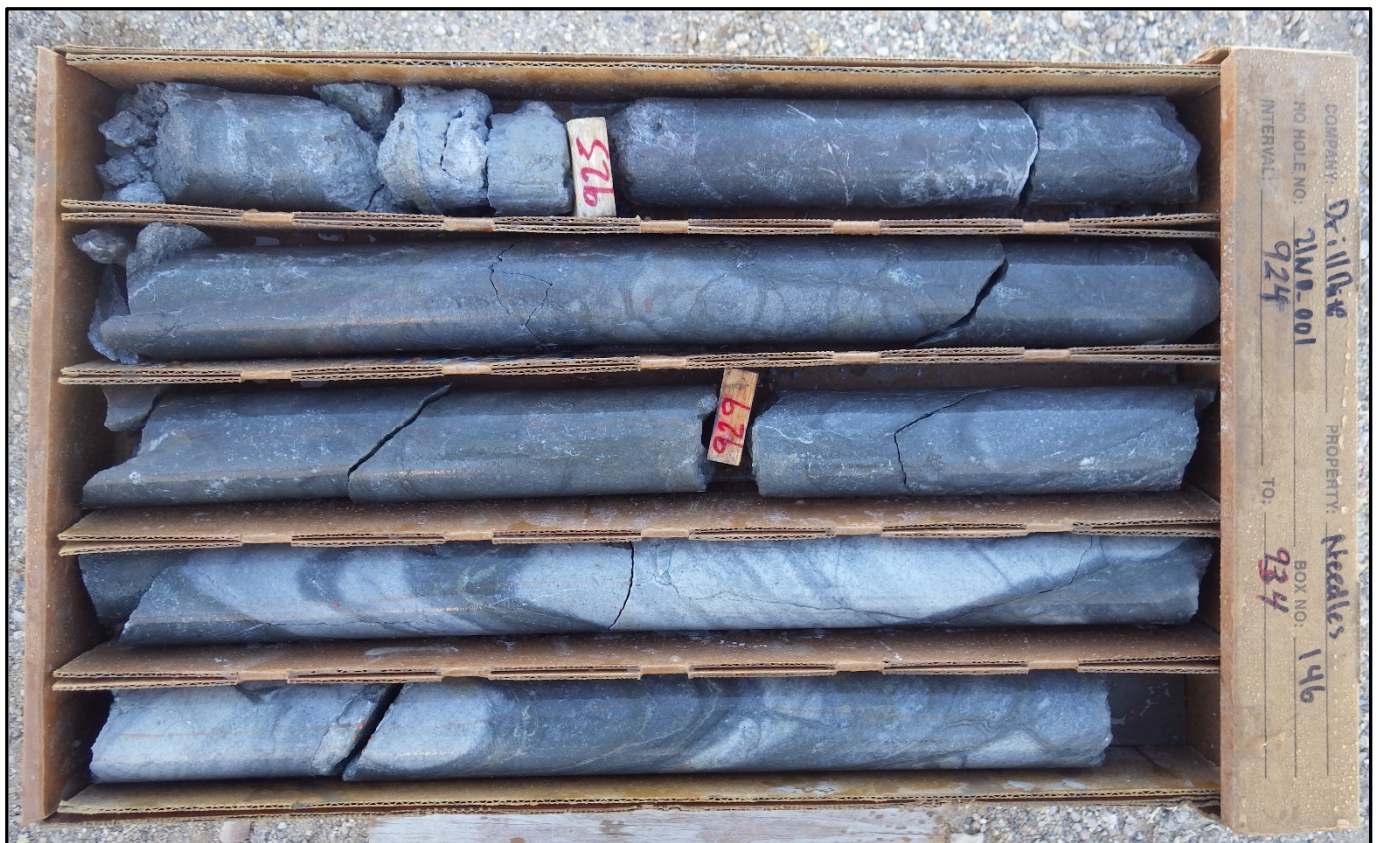
Figure 5. Core photo from 924ft to 934ft (281.6m to 284.7m) in hole 21ND_001 showing silicified and propylitically altered andesites containing disseminated and vein-hosted pyrite (dark grey).
