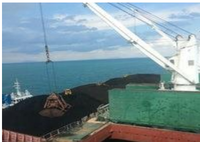
Coal being loaded from barges onto bulk carriers at the Taboneo Anchorage
