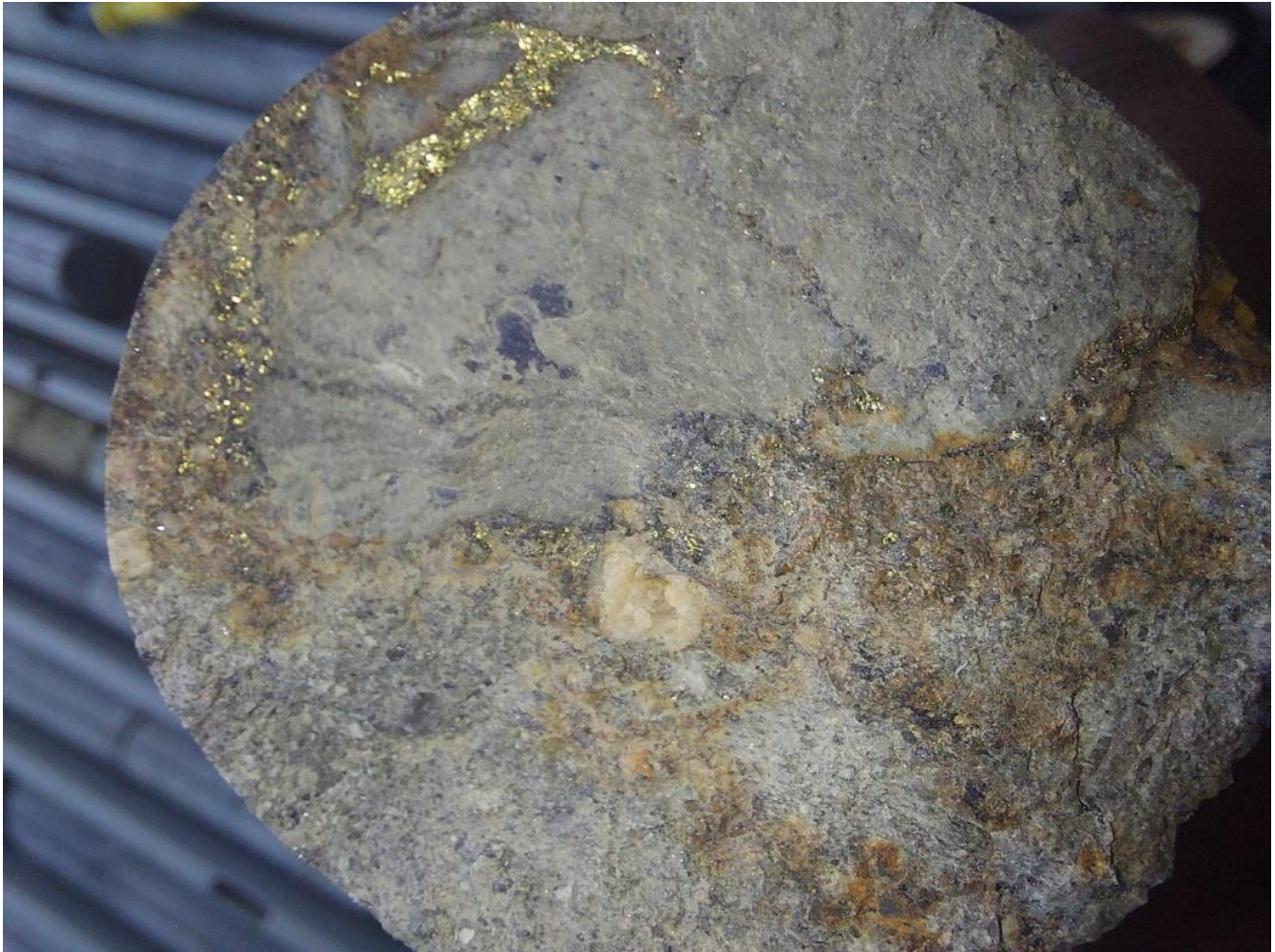
Photo 1: Nosib Prospect, end view of NSBDD003 drillcore at 83m with chalcopyrite and bornite mineralisation
