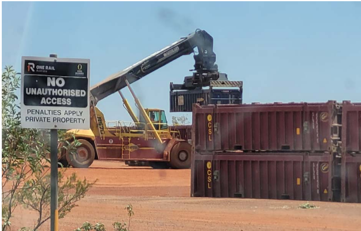
Linfox's Reach Stacker moving half-height sea containers in Tennant Creek similar to what will be used by Peko to unload trucks
