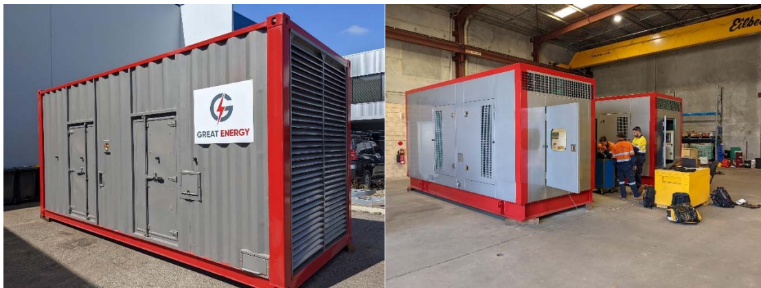
Three 500kVA Diesel Generator Sets Preparing to leave Elmore's Malaga Workshop
