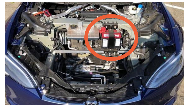
All commercially produced EVs have 12V lead-acid batteries
