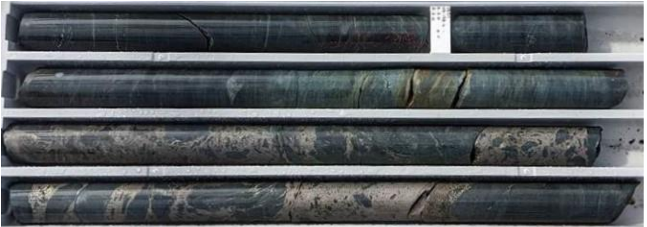
Figure 1. Matrix to semi-massive sulphide mineralisation in JD211.
