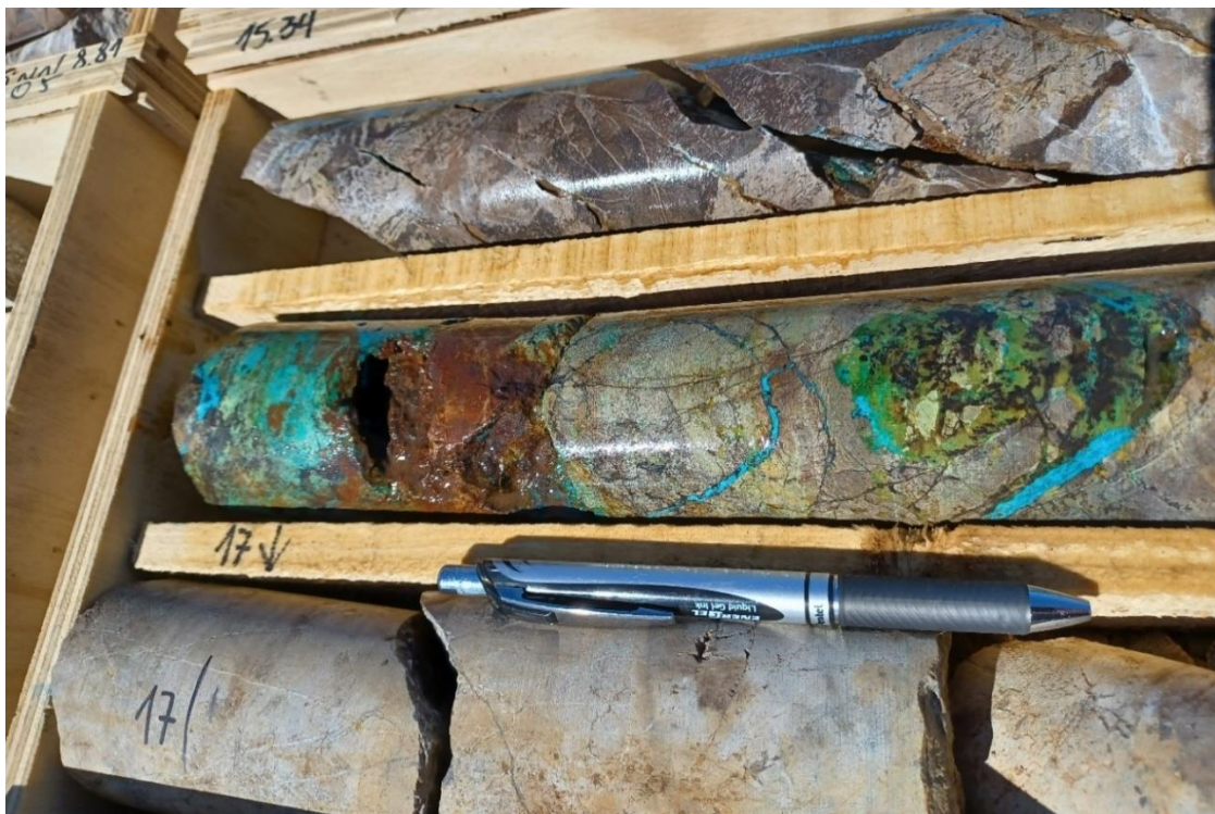
Figure 1: Visual copper mineralisation (malachite and chrysocolla) intersected in drillhole CMPDD006 at 16m downhole. The Company notes this is based on a visual inspection only and the samples are yet to be assayed or analysed.
