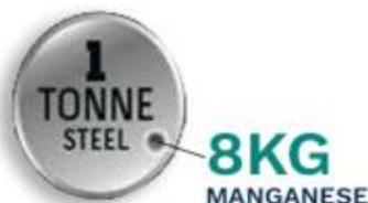
AVERAGE AMOUNT USED IN STEEL FOR STRENGTH, HARDNESS AND ABRASION RESISTANCE
