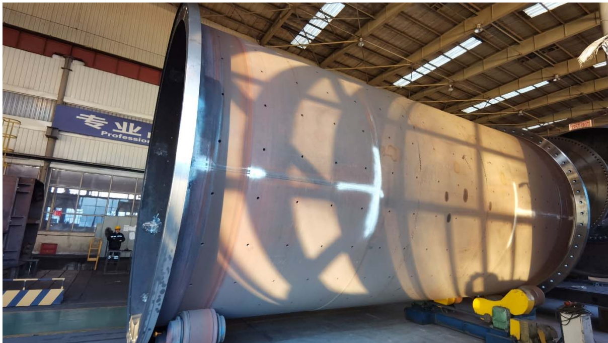
The Ball Mill Shell During Construction
