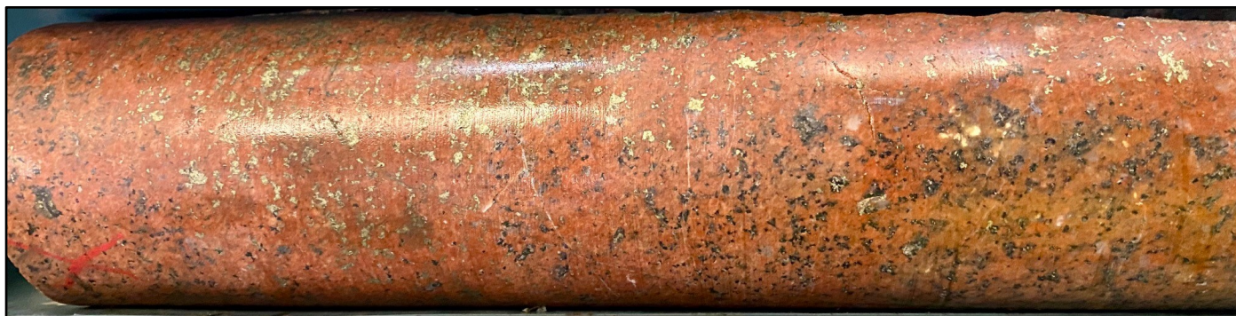
Figure 7. Disseminated chalcopyrite in pervasive potassic altered granite around molybdenite filled fracture (149.4m)
