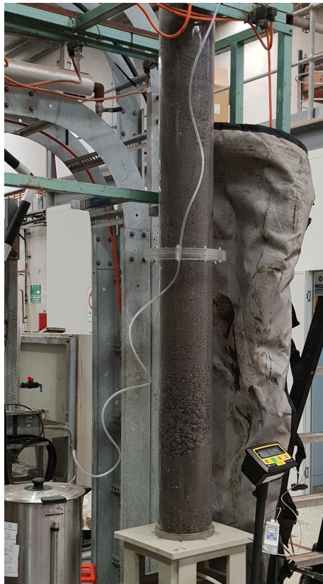
Image 3 / Nifty Metallurgical Column Test Work
