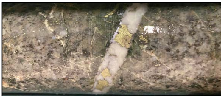
Figure 6. Chalcopyrite and molybdenite bearing quartz vein with discrete alteration halo (48.6m)
