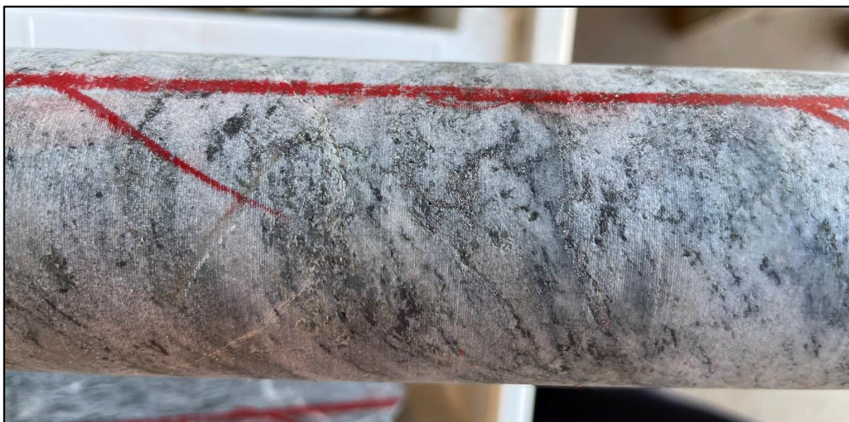
Figure 3A: Angepena Prospect – NQ diamond drill core (48mm diameter) showing intensely bleached, carbonate-altered dolerite.
