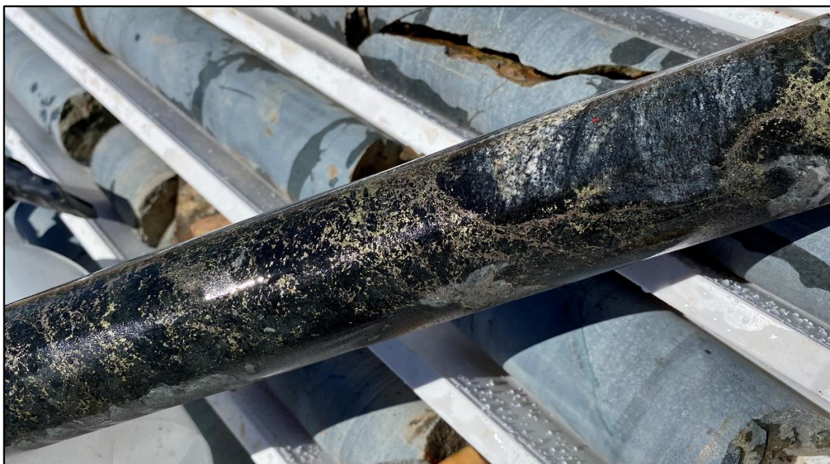
Figure 3B: Angepena Prospect – NQ diamond drill core (48mm diameter) showing dolerite-hosted chalcopyrite and pyrrhotite.
