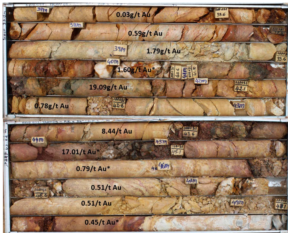
Image 1: Pranoi Prospect - photo of diamond core from DDD0031 37-49m oxidized showing altered sediments with obvious quartz veins and ferruginous zones with meter gold grades. This shows part of the intercept 12m at 4.48g/t Au from 38m.
