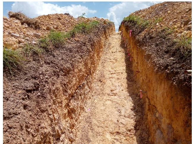
Images 2 and 3: Trench GCH2-TR01 single trench excavated to provide preliminary assessment of the gold-in-soil anomaly returned very encouraging results of 20m @ 1.02g/t Au including 9.0m at 2.06g/t Au.
