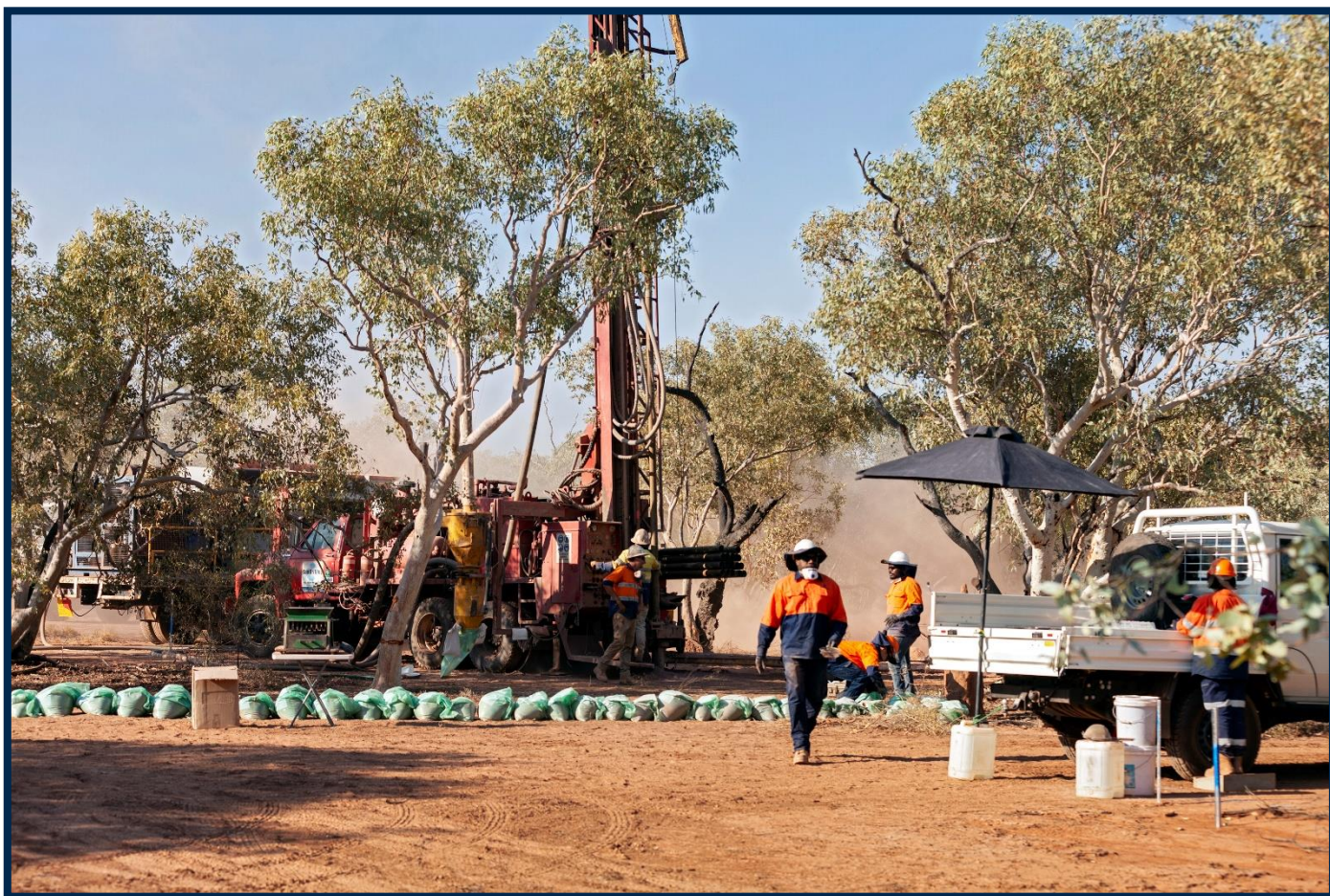
Photo 1: Reverse circulation drill hole (HERC003) in progress. Note sand cover and lack of surface expression.
