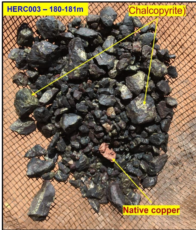
Photo 4: Reverse Circulation drill chips showing copper (chalcopyrite) in the deeper primary of drill hole HERC003.
