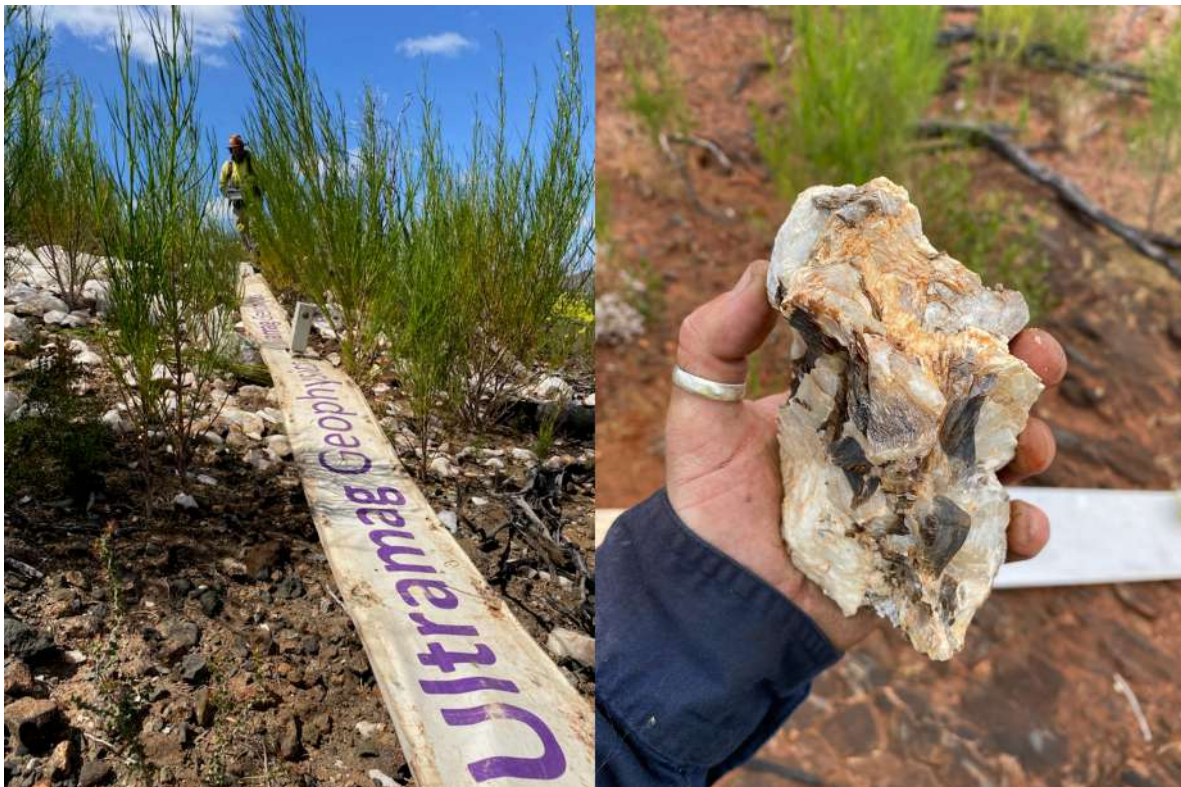
Figure 2: DGPR surveying and coarse-grained, prospective coarse-grained pegmatite from outcrop
