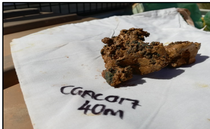
Figure 4: Nickel laterite mineralisation, CGAC017, 40m depth (White Cliff Minerals, 2018 aircore drill programme)
