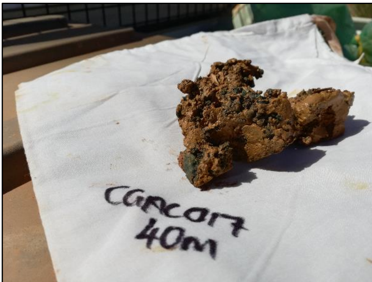
Figure 10 Nickel mineralisation, CGAC017, 40m depth (White Cliff Minerals, 2018 AC Program).
