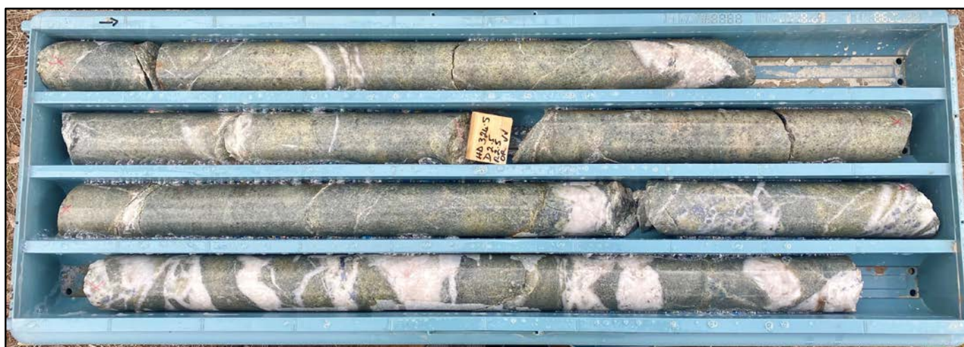
Figure 7. Abundant quartz veining and brecciation in intense sericite alteration (21TVDD001, 323.1m – 326.6m).
