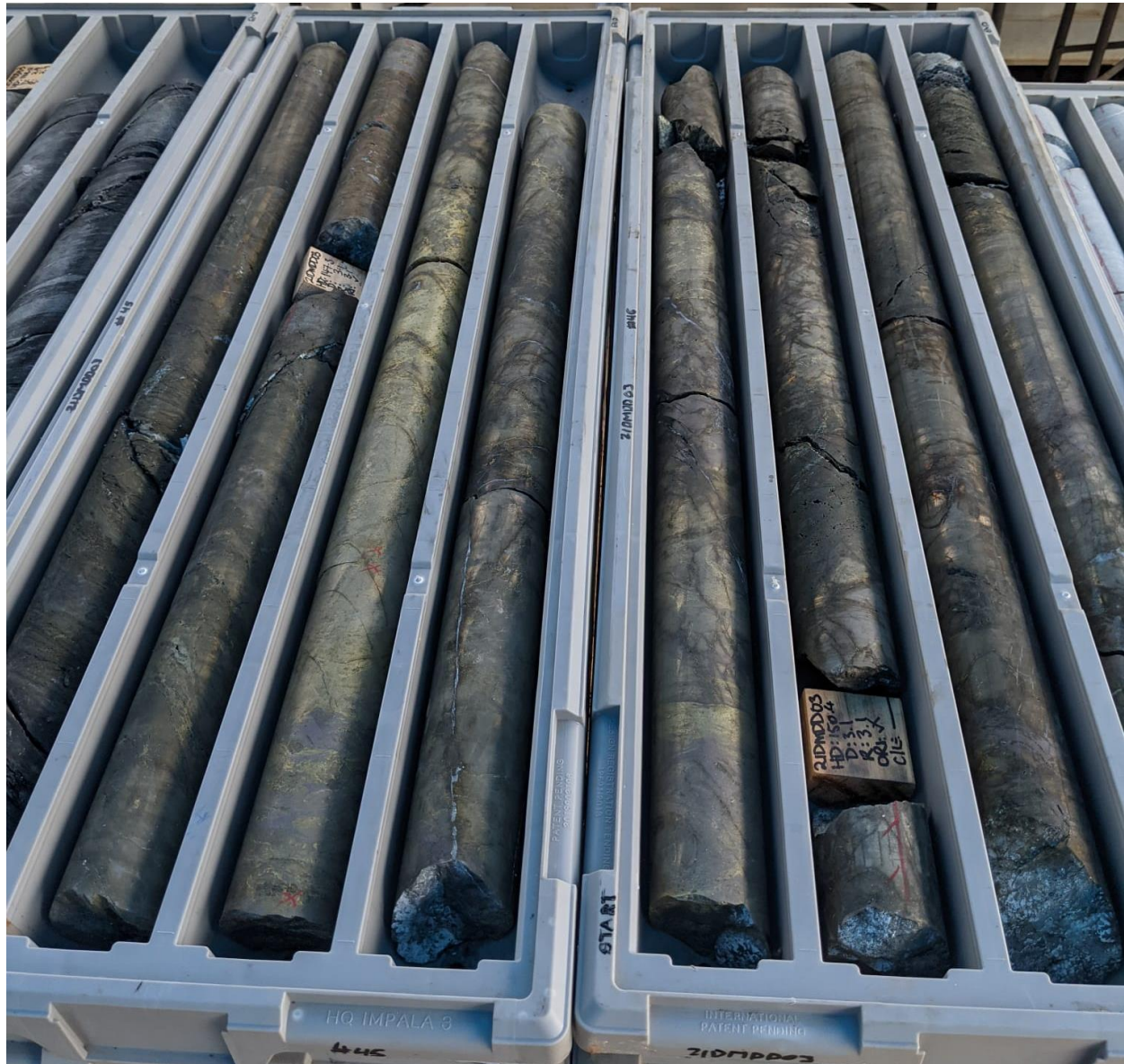
Summary Image 2 – Revolver Drill Hole 21DMDD03 Massive Sulphide full core sample.
