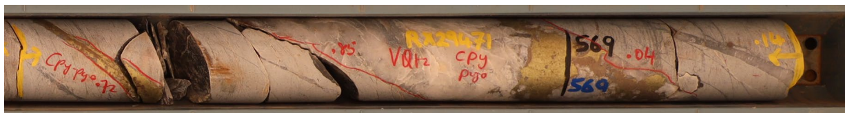
Figure 1. NQ core from diamond hole MFED095 with chalcopyrite - quartz veining in the sediment footwall adjacent to the Musket nickel deposit. This sample interval of 568.69 - 569.14 metres downhole returned 4.23% copper and 161.1 g/t silver.
