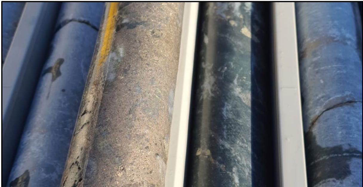
Figure 1. Semi massive and disseminated sulphide intersected by NDD0010 around 140m downhole. The hole size is NQ2.
