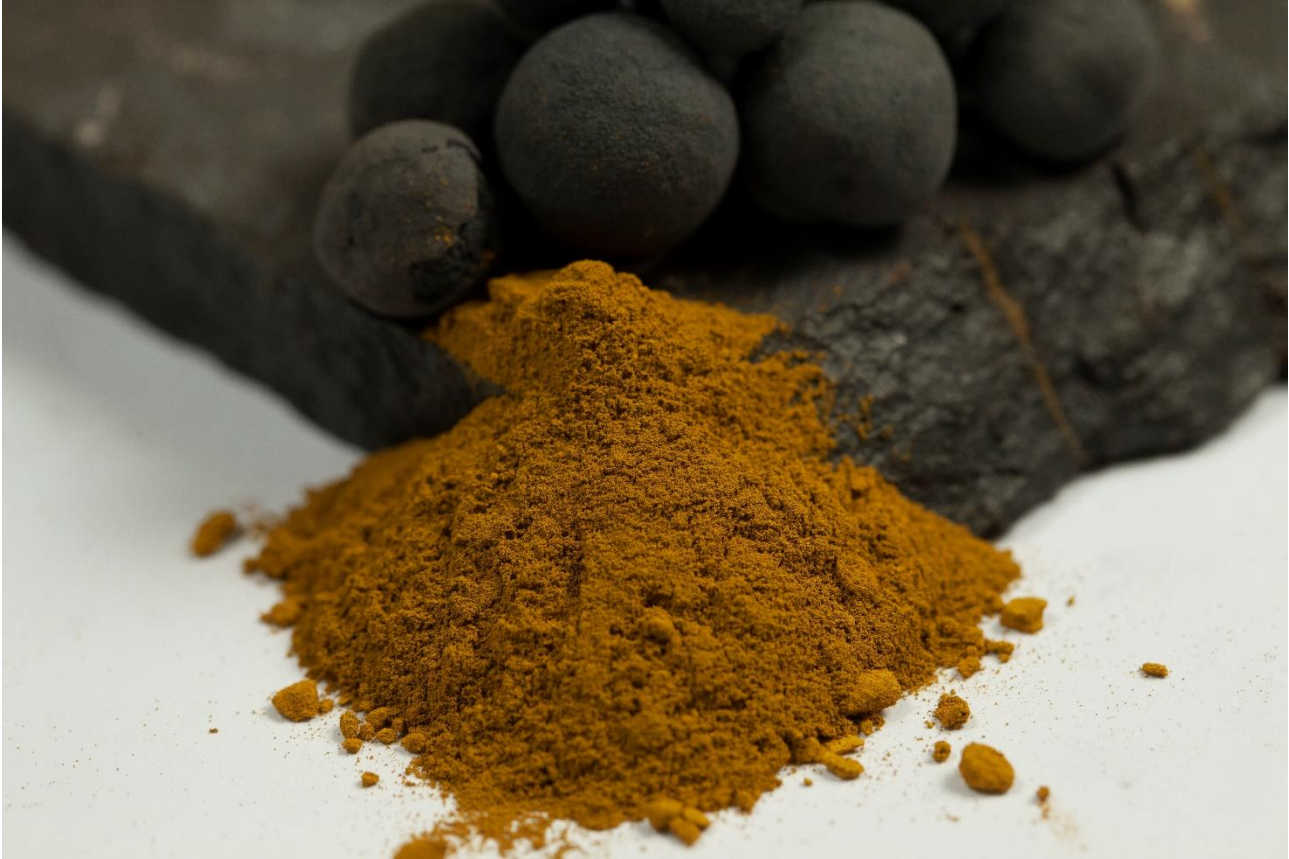
Figure 1. Sample of V_2O_5 precipitate generated from pilot program alongside roasted pellets and a vanadium ore sample.
