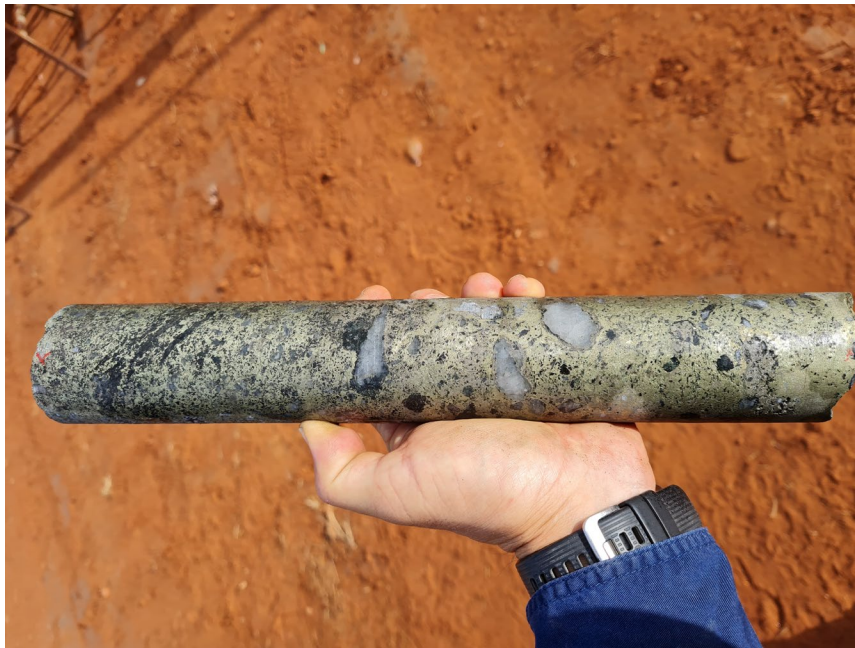
Figure 2. Photo of breccia copper mineralisation from NLDD042.
