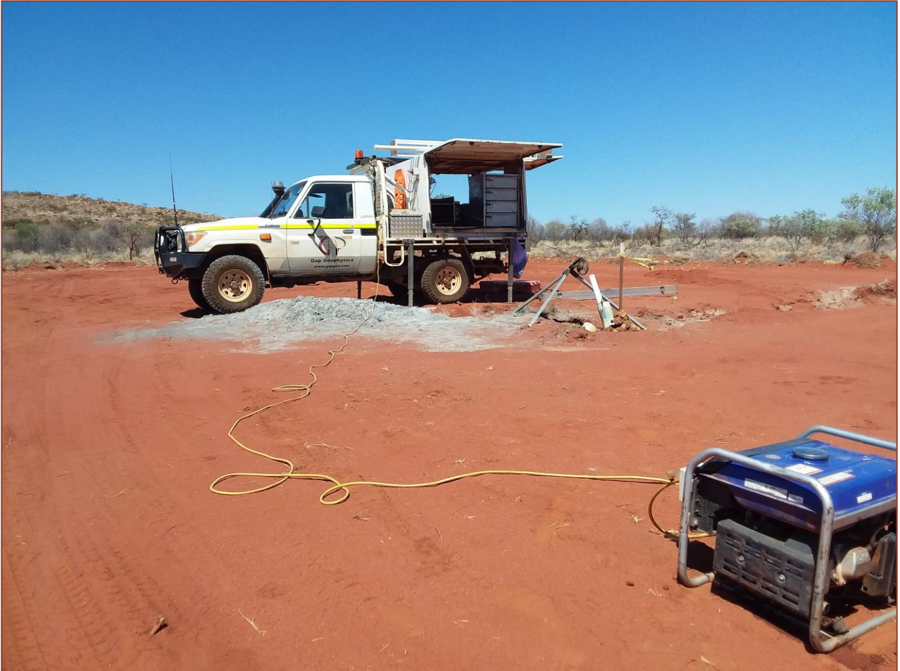
Figure 1: Downhole Electromagnetic Survey (DHEM) underway at Victoria Bore
