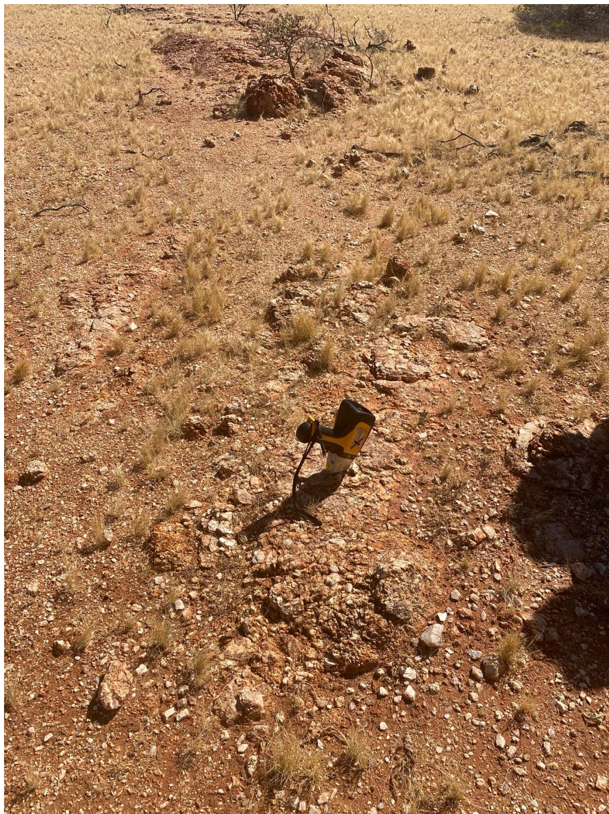
Figure 10: Yinnetharra Pegmatite E09/2628. Completing Handheld XRF readings on typical low relief pegmatite outcrop.
