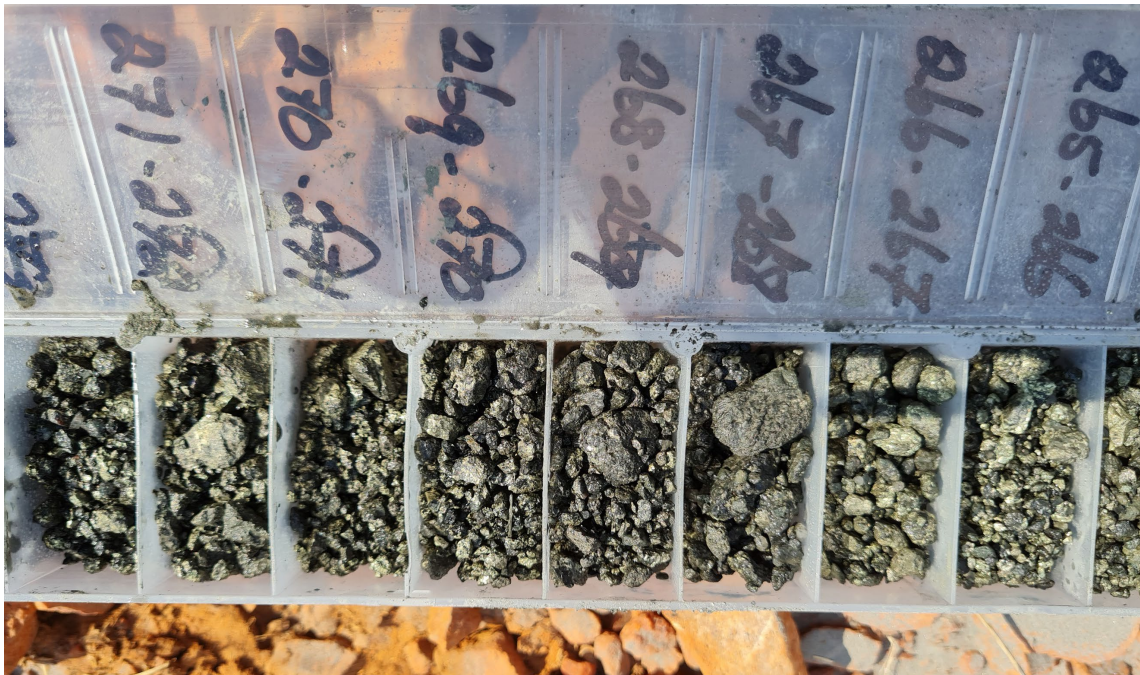
Figure 3. Photo of RC drill chips from NLDD044 showing intervals of semi massive copper sulphide mineralisation.
