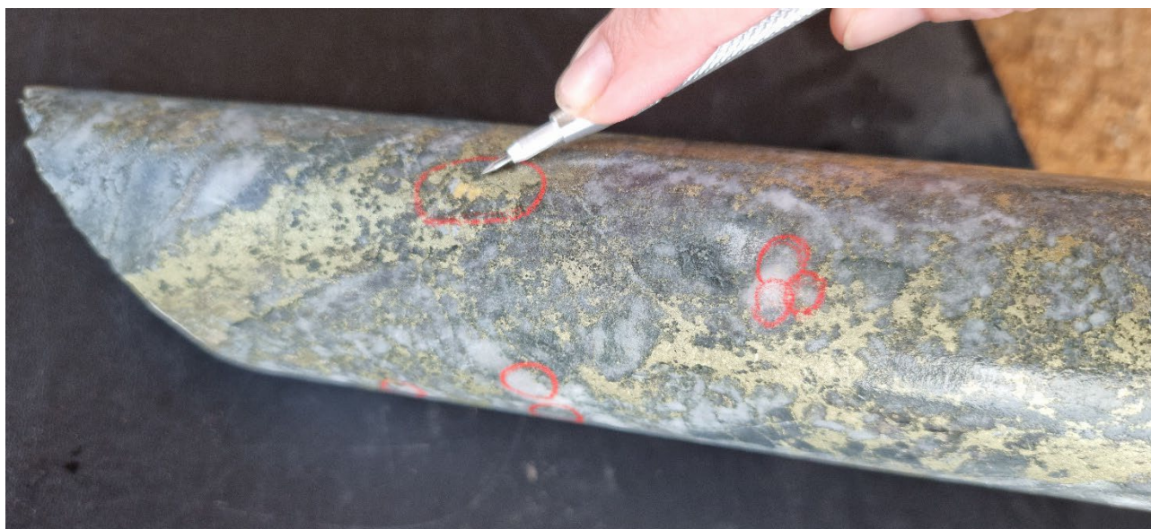
Figure 5: DD21KP1033 showing multiple fine gold particles of visible gold (circled red) at ~ 102m down hole.
