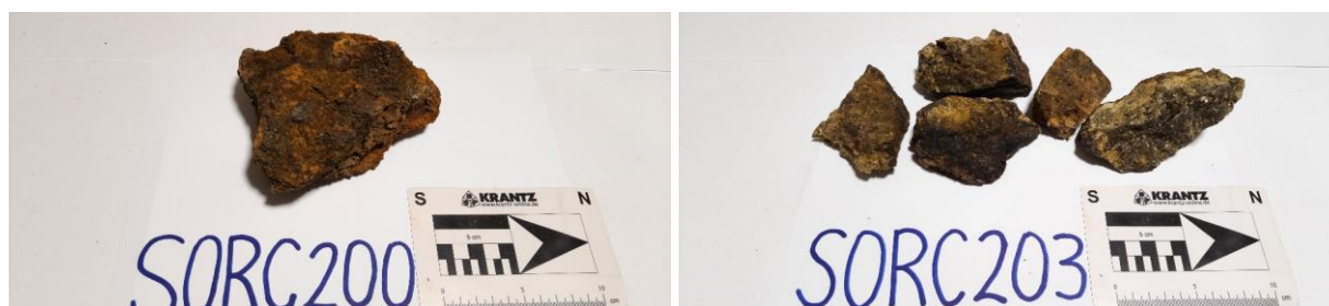
Figure 2: Samples SORC200 which returned 458ppm Co and 0.22% Ni and sample SORC203 which returned 524ppm Co and 0.45% Ni
