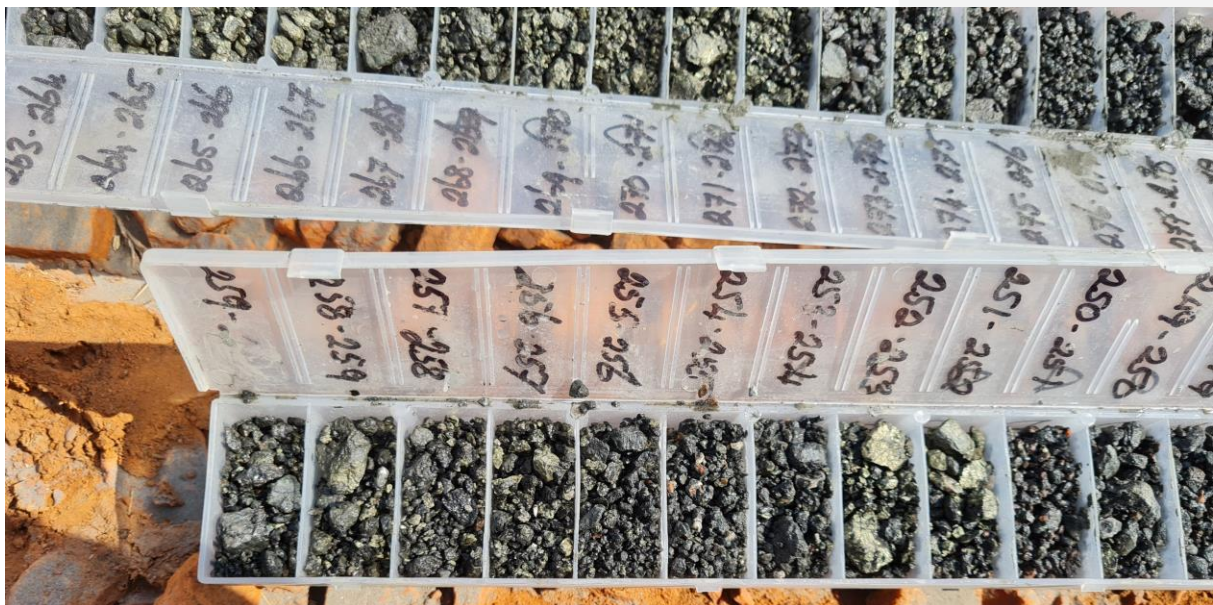
Figure 4. Photo of RC drill chips from NLDD044 showing intervals of semi massive copper sulphide mineralisation.
