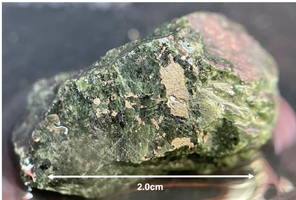
Photo 3: Poly-Phased Sulphides in 21BHRC002 (dominant sulphide is Pyrrhotite with minor Chalcopyrite) from 278 to 279m downhole
