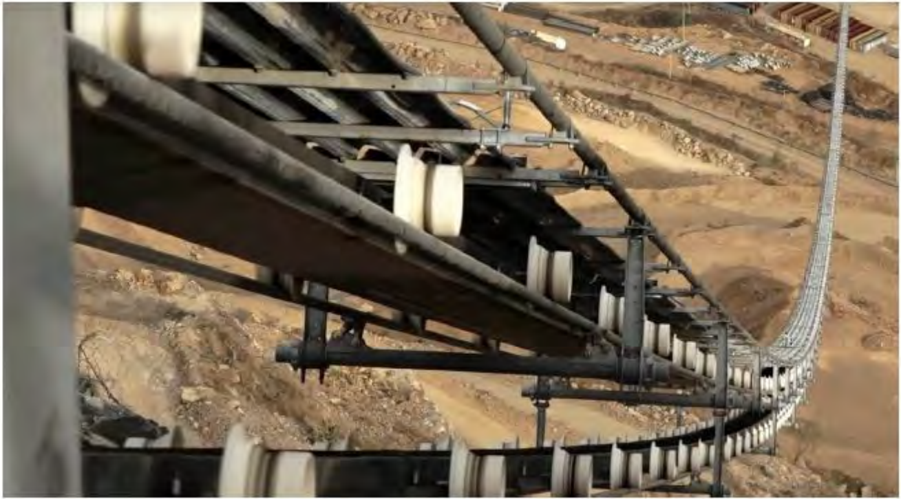
Figure 30 Close-up view - RopeCon transports material on a flat belt with corrugated side walls that is fixed to axles that run on track ropes suspended from tower structures.
