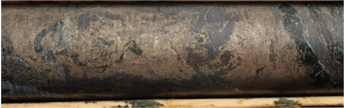
Figure 6: DDED21-059: semi-massive (pyrrhotite-pentlandite-chalcopryrite) within fine grained sheared peridotite at contact with rhyolitic tuff at 54.5m (dry core)
