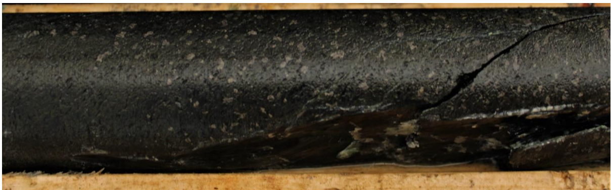
Figure 8: DDED21-059: Coarsely disseminated sulphide (pyrrhotite-pentlandite) 5% within medium grained peridotite from 180.5m
