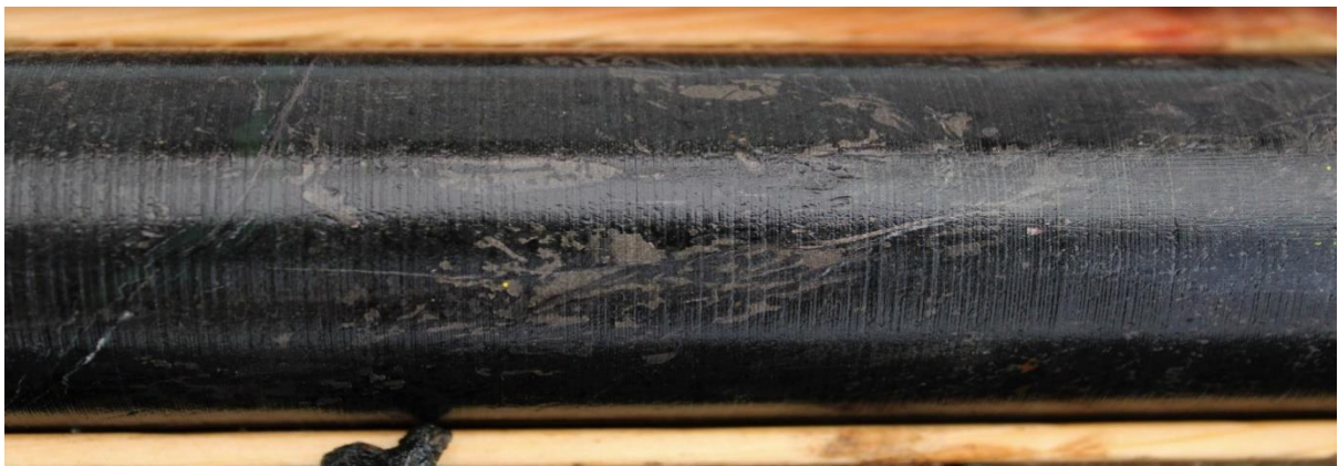
Figure 7: DDED21-059: blebby (pyrrhotite-pentlandite) 5% within fine grained peridotite at 86m
