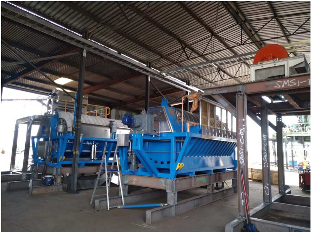
Two ceramic disk filters, each with a magnetic separator – these units will de-water the final magnetite concentrate prior to it being loaded into half height sea containers to be sent to port
