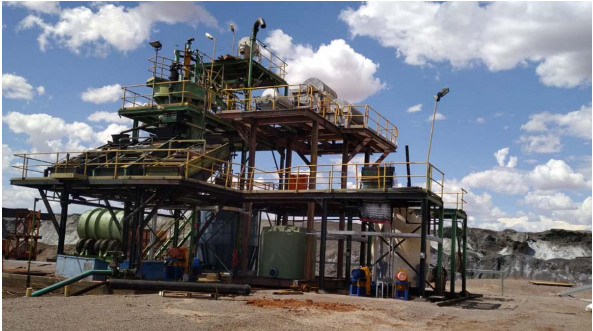
Process plant with magnetite tailings stockpile in the background Photo includes scrubber (background left) mixing tanks (ground level), multiple magnetic separators, cyclones and Derrick screens (elevated)
