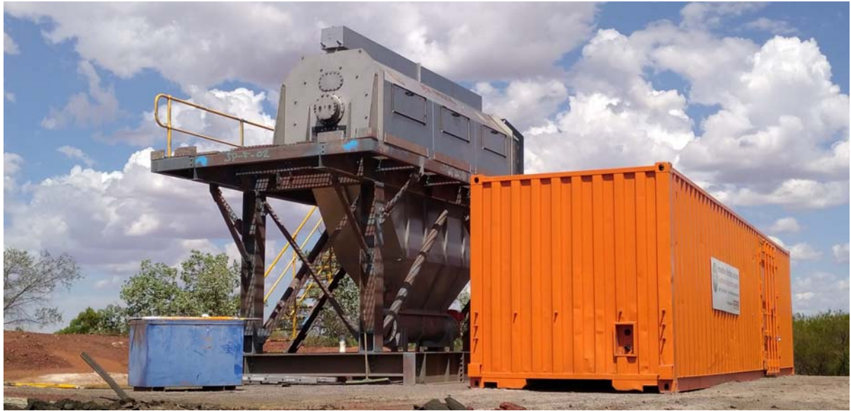
Screw press and screw press control room – used for dewatering tailings
