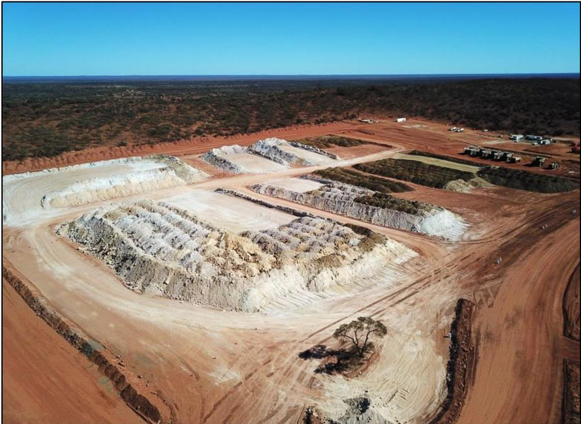
**Figure 11 | Ore mined from the Bungarra open pit stockpiled on the NLGP ROM**
