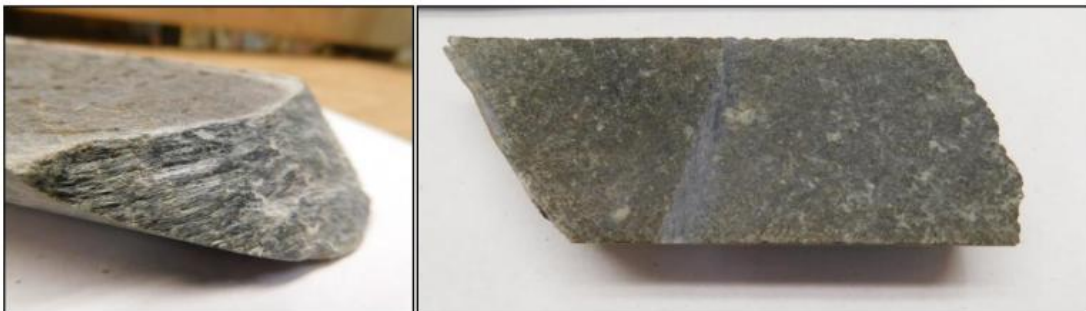
Left: Sample of massive holmquistite showing asbestiform habit (hole 17-BD-54, 94.73–94.90 m). Right: Sample of amphibolite with vein of blue-colored holmquistite (hole 17-BD-82 94.49–94.59 m).
