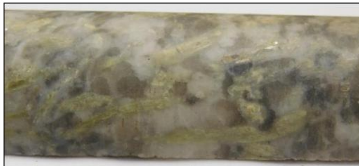
Figure 6-4. Pegmatite showing Pseudomorphs of Muscovite after Spodumene (Hole 17-BD-121 72.24–72.44 m)
