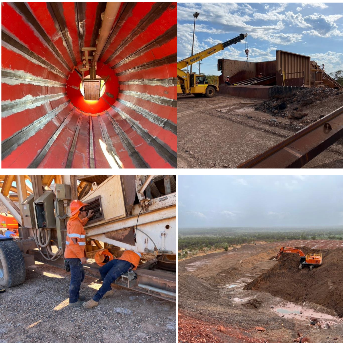
Figures 5-8. Interior of the crushed ore agglomerator, which has been re-lined in preparation for operation, replacing feed bin grizzly bars, adjusting sensors on stacker, and re-mining heap leach ore.
