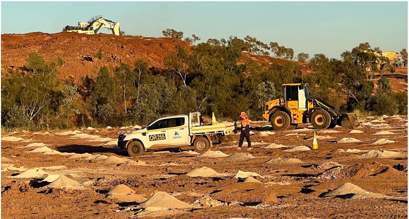
Figure 3. Whilst mining is underway at Anthill east pit (top left), adjacent benches have been drilled and loaded for firing.
