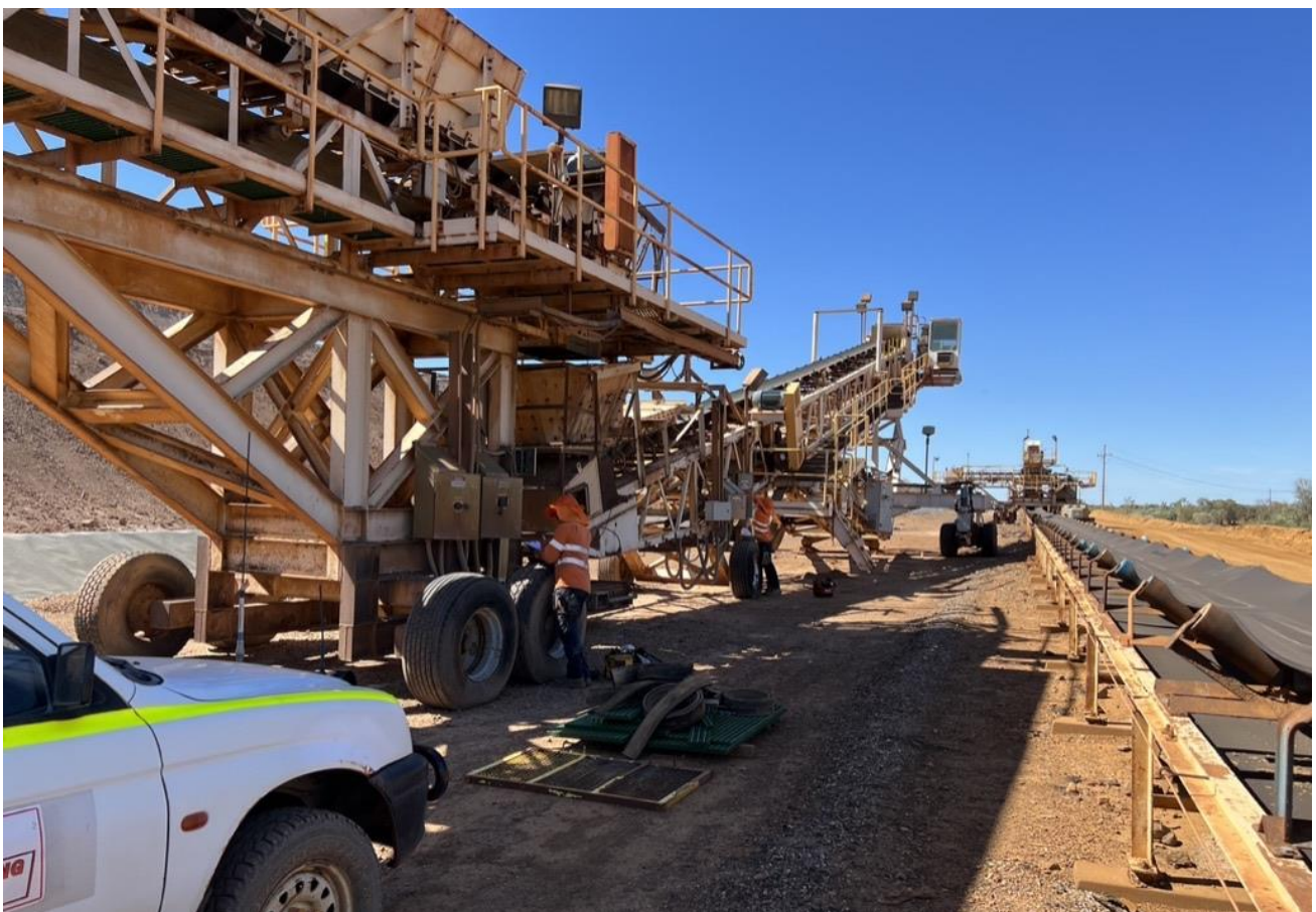
Figure 4. At Mount Kelly, the heap leach stacker being refurbished in preparation for test commissioning of the crushing and stacking circuit.
