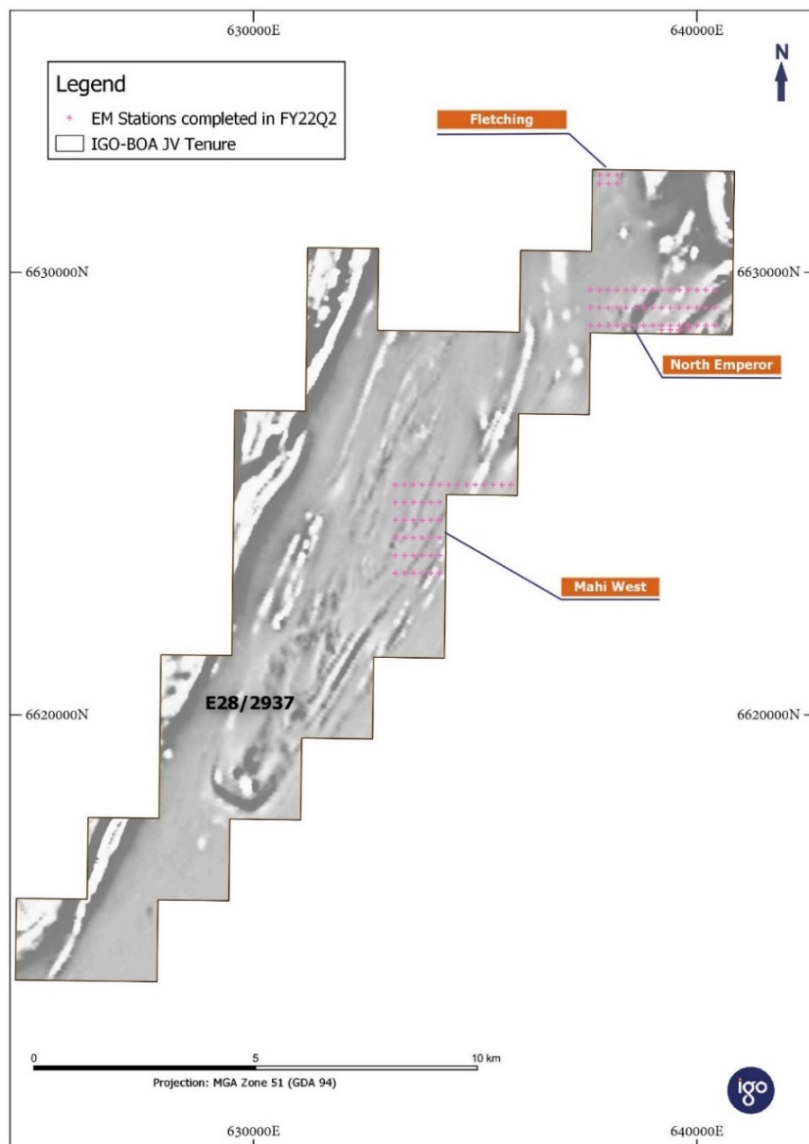
Figure 2 Completed MLEM stations in FY22Q2 on E28/2937, overlaying the First Vertical Derivative (1VD) of an airborne-derived Total Magnetic Intensity (TMI) Reduced to the Pole (RTP) image
