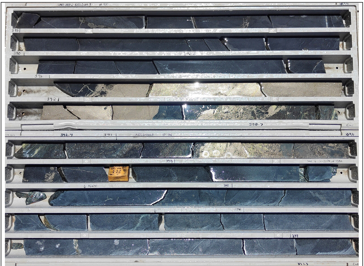
Figure 2: AELD0003, NQ2 drill core showing massive sulphide zone (391.04 – 393.76) and adjacent zones which exhibit high competency (solid core) and high recoveries. The core competency and lack of talc-chlorite shearing augurs well for good mining ground conditions. Note the down hole depth metre marks shown in black on the core trays.
