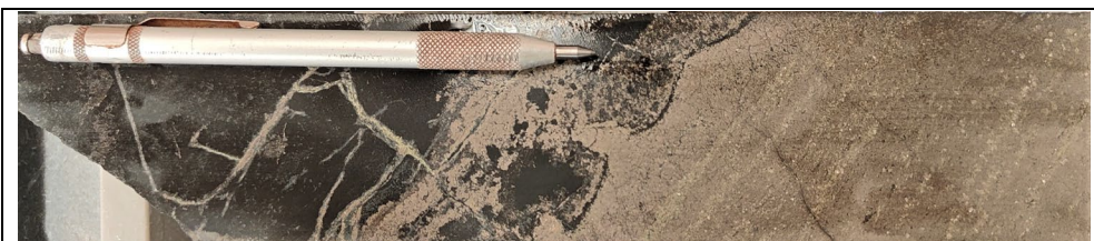
Figure 1: AELD0003, NQ2 drill core from 391.04m showing the dacite footwall contact and thermal erosion on the left hand side of the photo and high grade massive nickel sulphide on the right hand side of the image.
