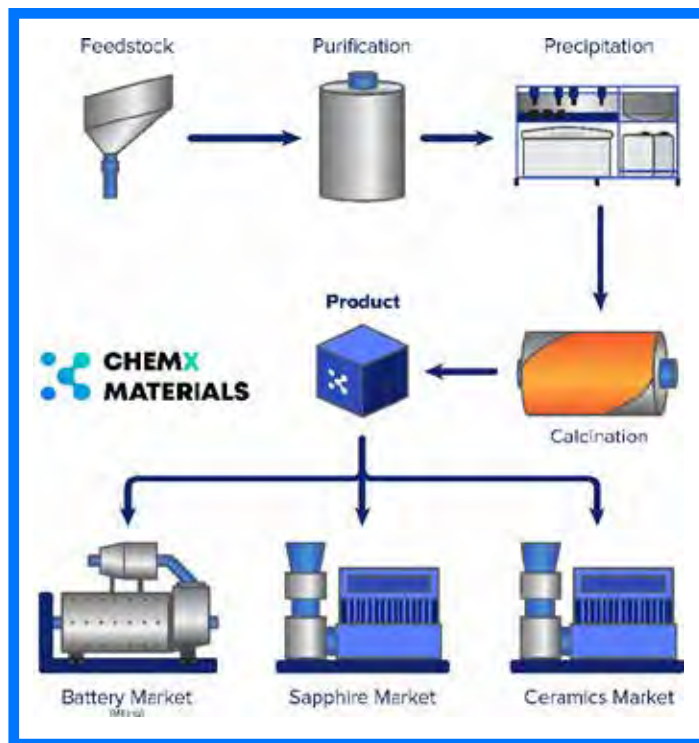
Diagram: ChemX 'HiPurA' High Purity Alumina (HPA) Flowsheet
