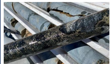
Chalcopyrite-pyrrhotite rich drill core from Angepena prospect at Moora
