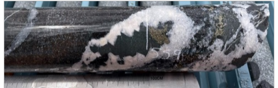
GDRCD007 - 559m, example of a quartz-calcite vein in altered diorite with pyrite ± chalcopyrite, chlorite "Jigsaw" infill and minor brecciation.
