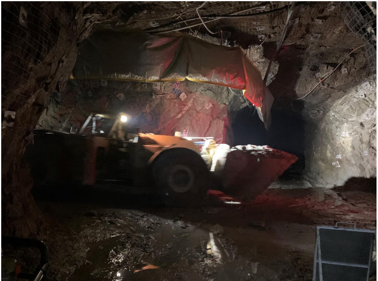
Figure 2: Loader transporting high grade ore at the A1 Mine
