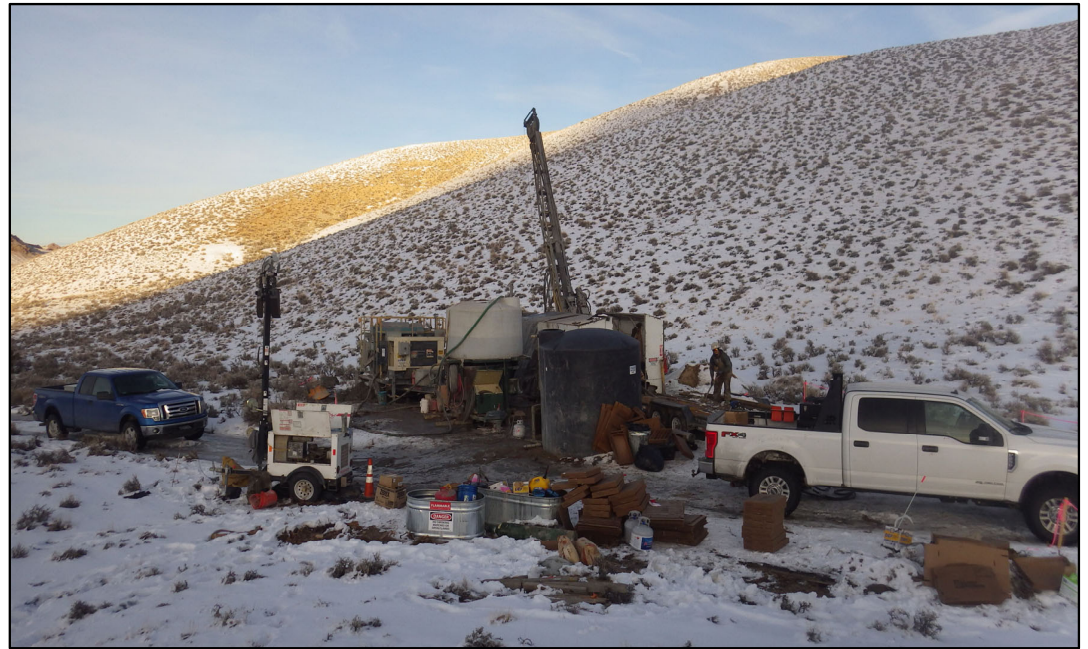
Diamond drill-rig sited over hole 21ND_002 (view to the northeast with the rig drilling toward the chargeability anomaly)
