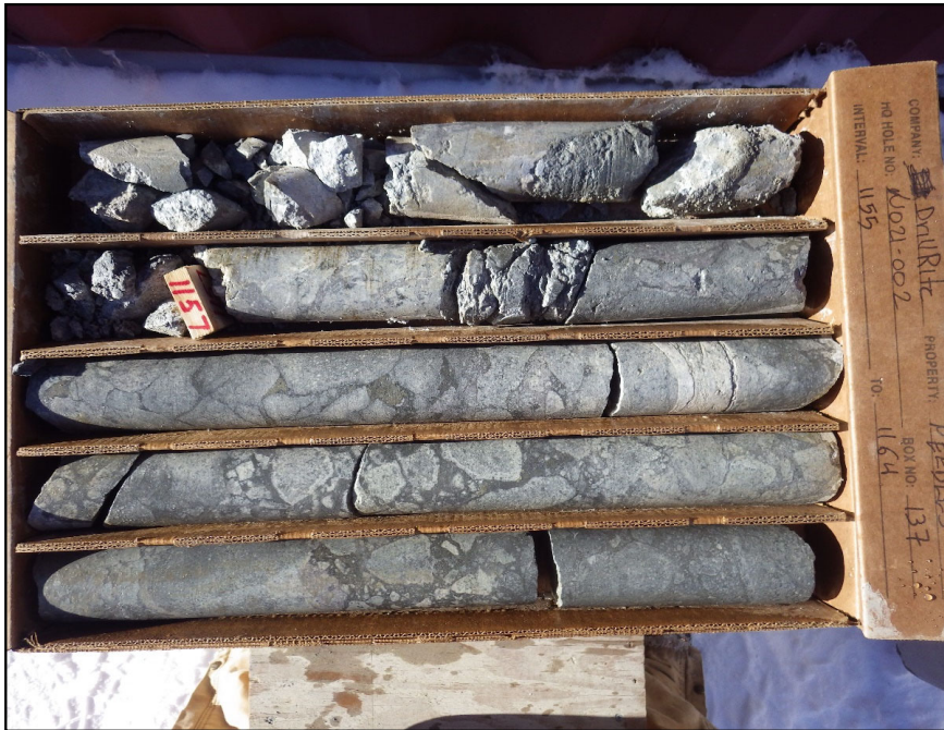
Brecciated unit in hole 21ND_002 showing altered andesite clasts within a pyrite-rich matrix (from 1155 to 1164ft (352 to 354.8m))
