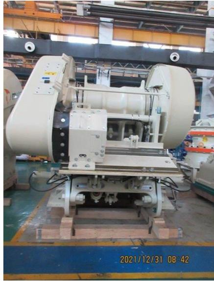
**Figure 2** – Manufactured Abra primary Jaw Crusher assembly.
