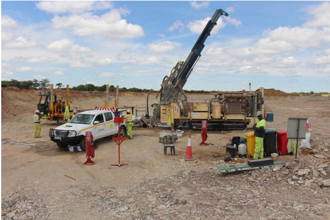
Figure 7. Grade Control Drilling at the Pit in progress
