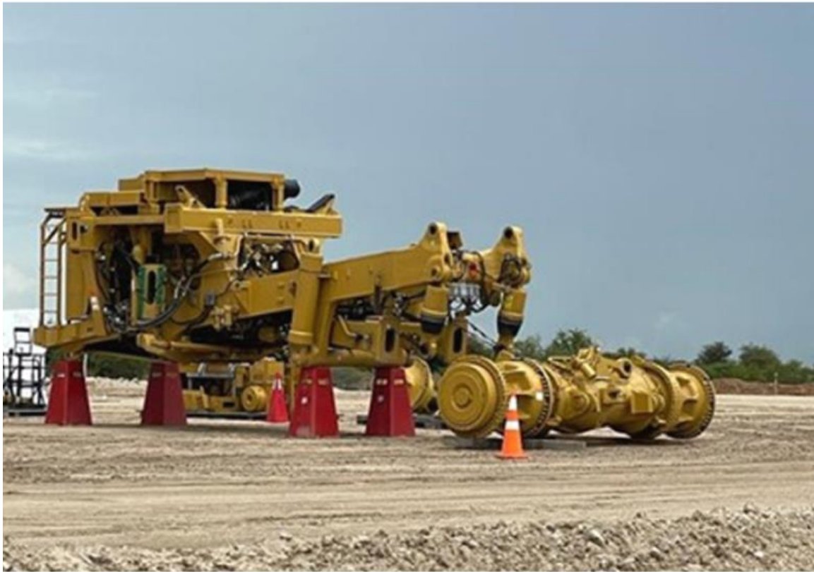
Figure 8. CAT 785 Dump Truck on Assembly Pad
