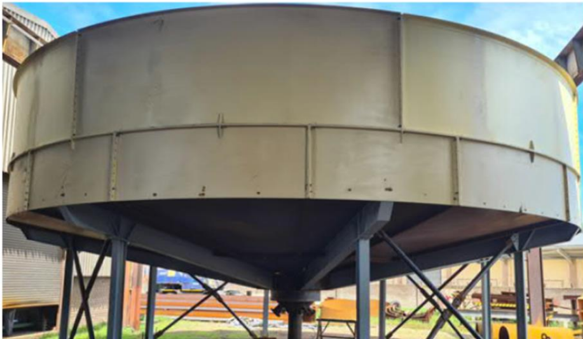
Figure 9. Concentrate Thickener trial assembly in South Africa
