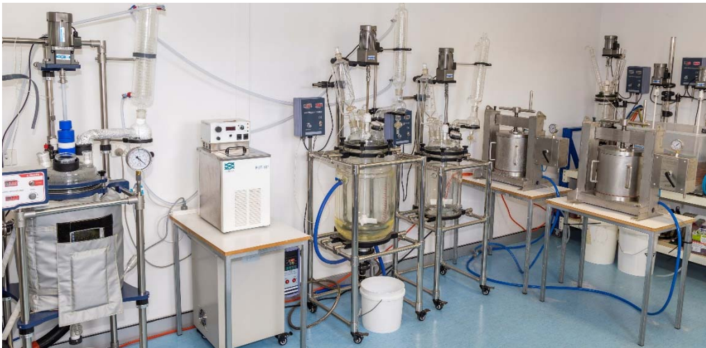
Figure 3: Laboratory Scale Pilot Plant – Type 1 Precursor production for market samples
