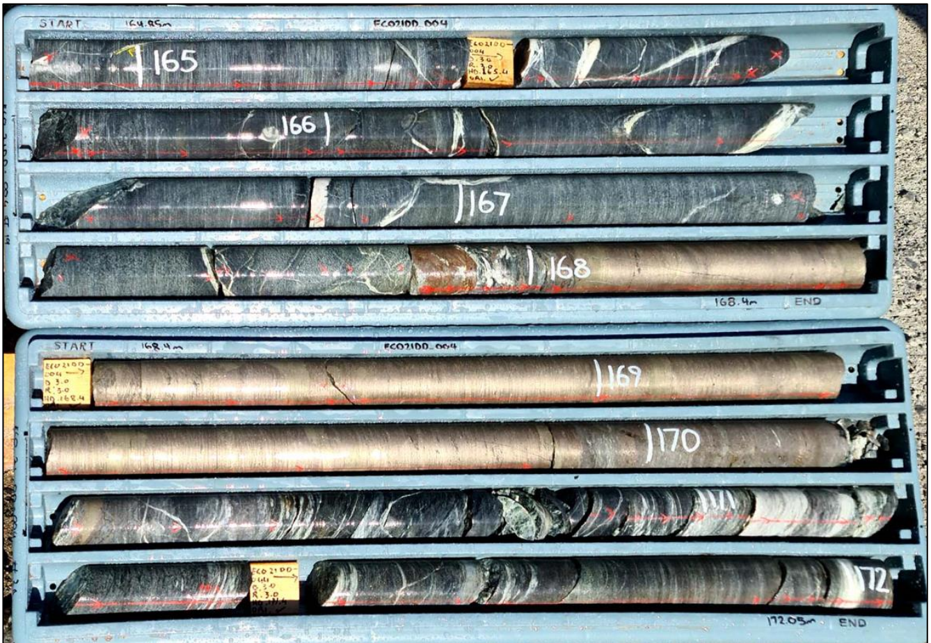
Figure 3 : Core from ECO21DD_004 - massive nickel sulphide zone from 167.85m downhole: 2.7m @ 10.72% Ni
