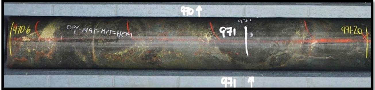
BOD059 – 0.6m grading 24.2g/t Au, 3.69% Cu from 970.6m – Chalcopyrite-actinolite-magnetite-hematite dusted albite hydrothermal breccia
