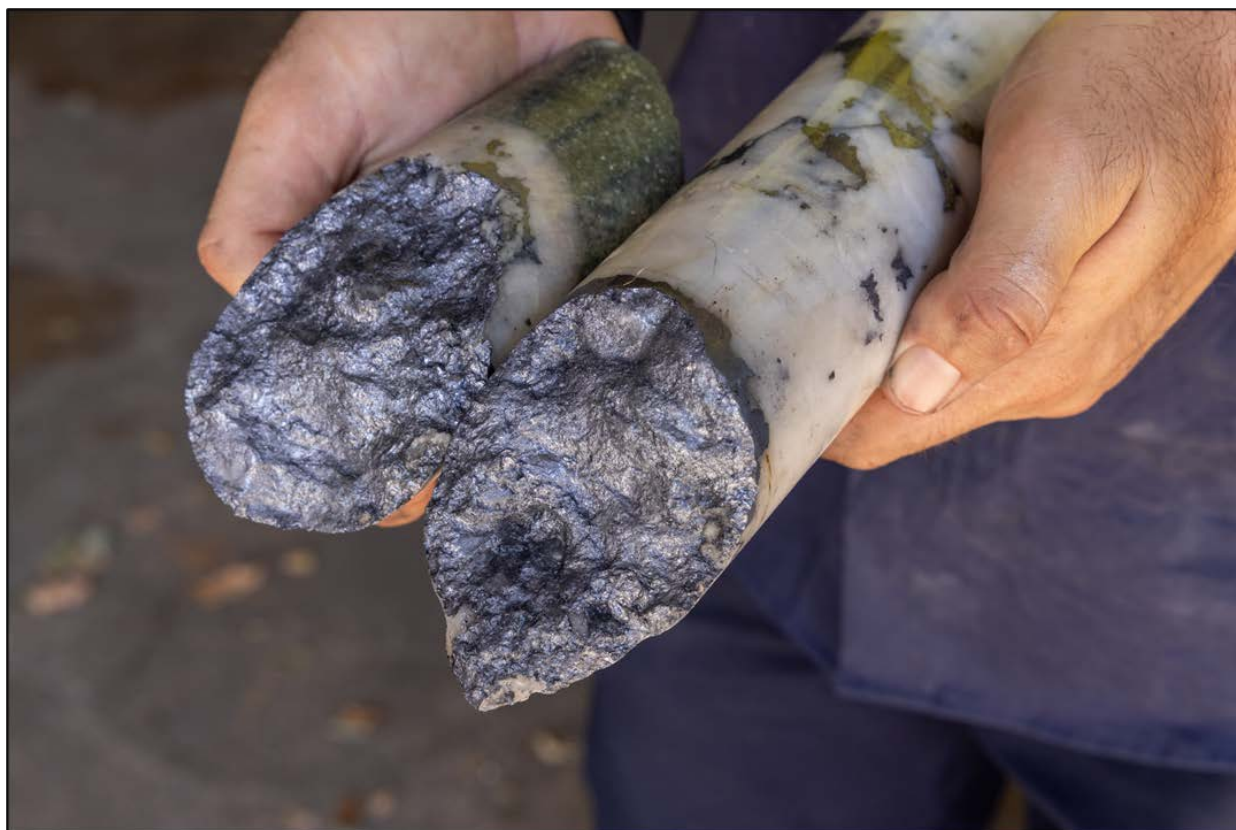
Figure 1. Molybdenite in quartz vein (338.1m, 21TVDD001).
