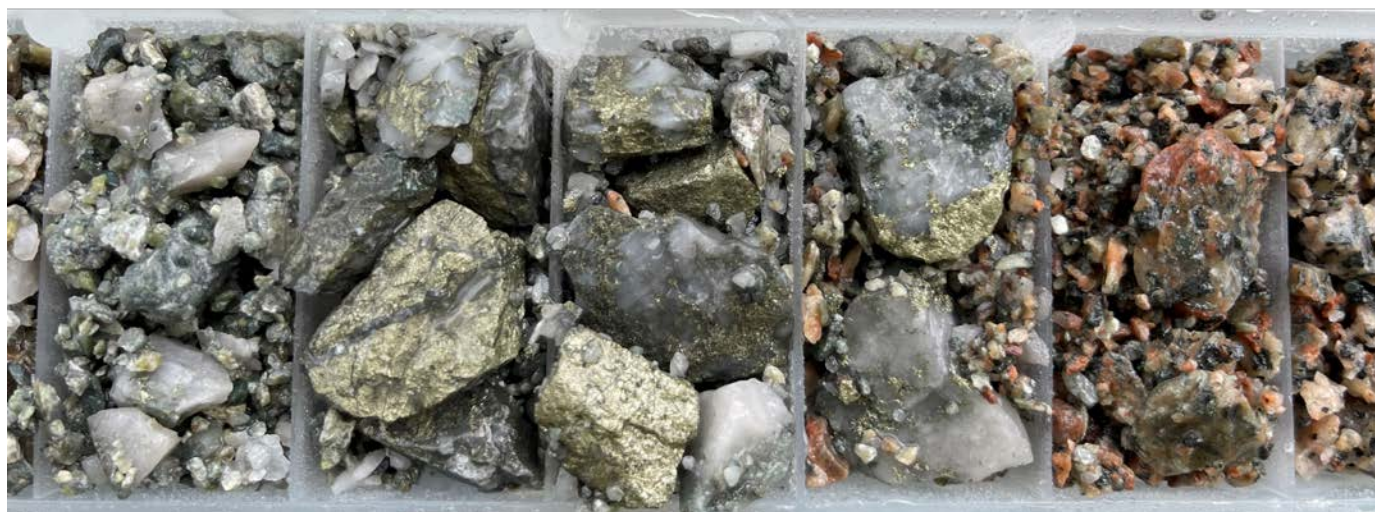
Figure 2. RC Chips containing chalcopyrite and molybdenite in 21KNRC004 (Kears).
