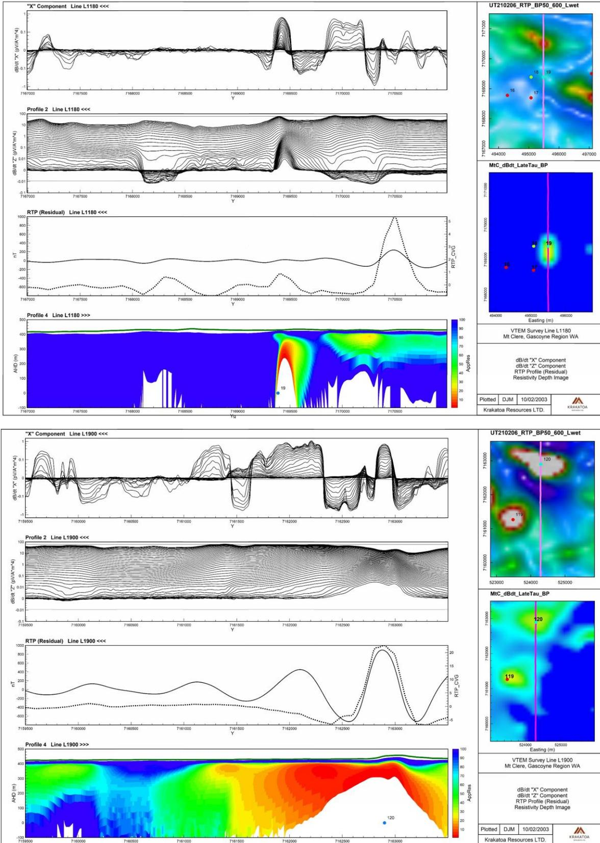
**Figure 5** Section plots through the Red Valley cluster - Line 1600 (top) and Dingo cluster - Line 1900 (bottom). Each Plot displays "X" and "Z" component observed data time decay profiles, Total magnetic field and derivative profiles (Reduced To Pole) with Resistivity Depth transform images. The equivalent profile length is displayed in plans over the residual Reduced to pole magnetic image and late time Tau image.
