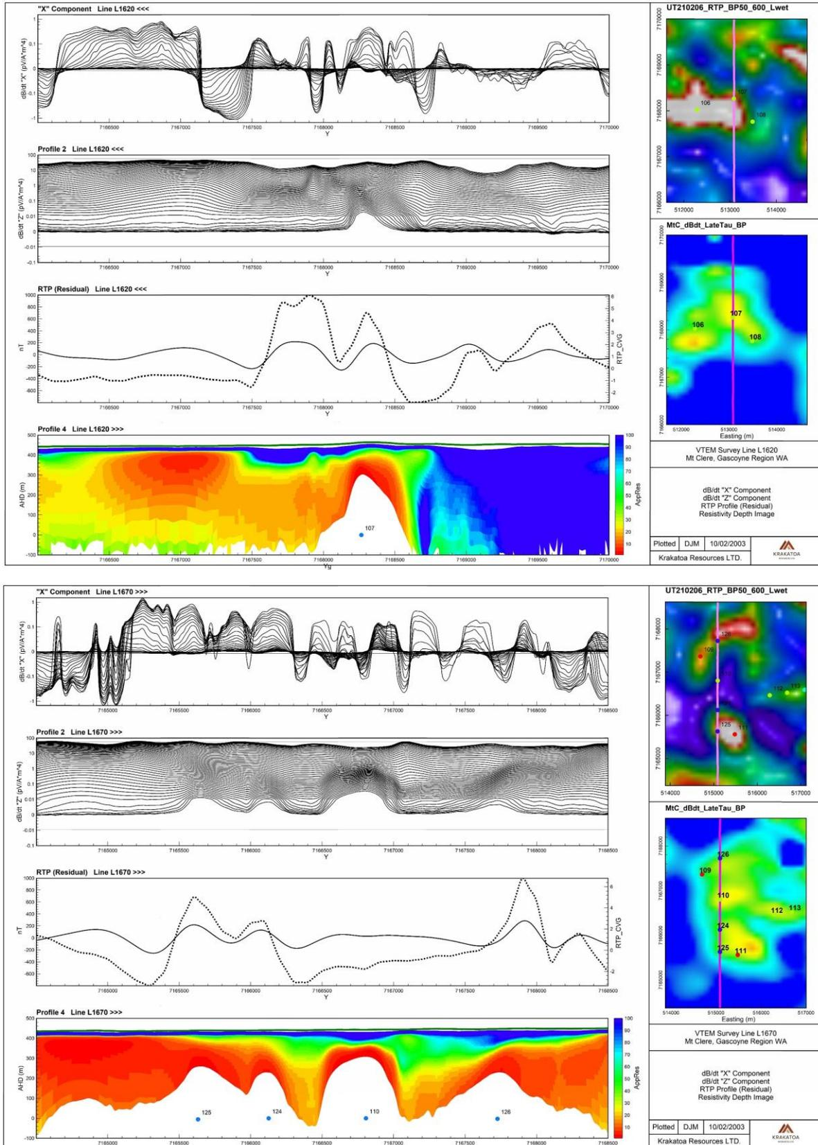
**Figure 4** Section plots through the North Bullbadger (NBB) cluster, showing Lines 1620 (top) and 1670 (bottom). Each Plot displays “X” and “Z” component observed data time decay profiles, Total magnetic field and derivative profiles (Reduced To Pole) with Resistivity Depth transform images. The equivalent profile length is displayed in plans over the residual Reduced to pole magnetic image and late time Tau image.
