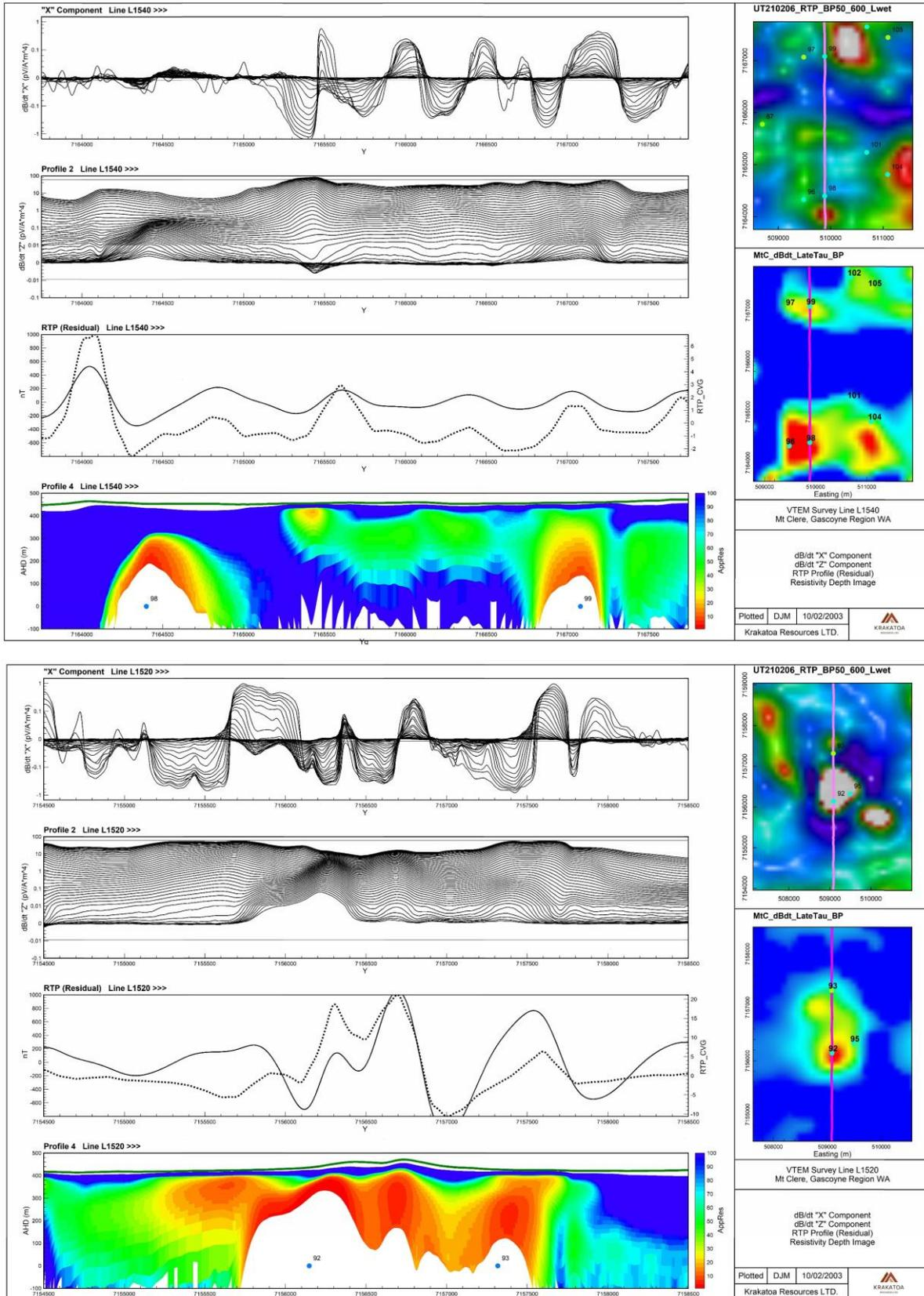
**Figure 3** Section plots through the Bullbadger cluster - Line 1540 (top) and Milly Milly cluster - Line 1520 (bottom). Each Plot displays "X" and "Z" component observed data time decay profiles, Total magnetic field and derivative profiles (Reduced To Pole) with Resistivity Depth transform images. The equivalent profile length is displayed in plans over the residual Reduced to pole magnetic image and late time Tau image.
